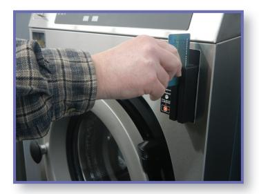
An external swipe is mounted on the face of most machines with wiring distributed through small holes provided during the installation. In place of the external swipe, some brands may require an external case and utilize a SmartLink style bezel with a display to be mounted on the top of the machine.
